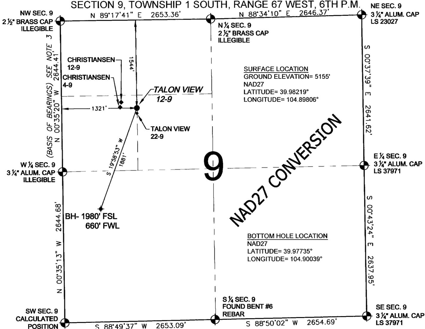
WELL TALON VIEW 12-9 TO BE LOCATED 1544' FNL AND 1321' FWL, SECTION 9, T1S, R67W OF THE 6th P.M.
