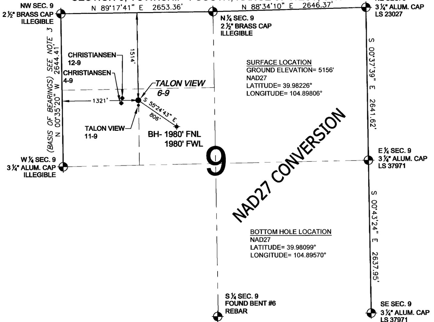
WELL **TALON VIEW 6-9** TO BE LOCATED 1514' FNL AND 1321' FWL, SECTION 9, T1S, R67W OF THE 6th P.M.
