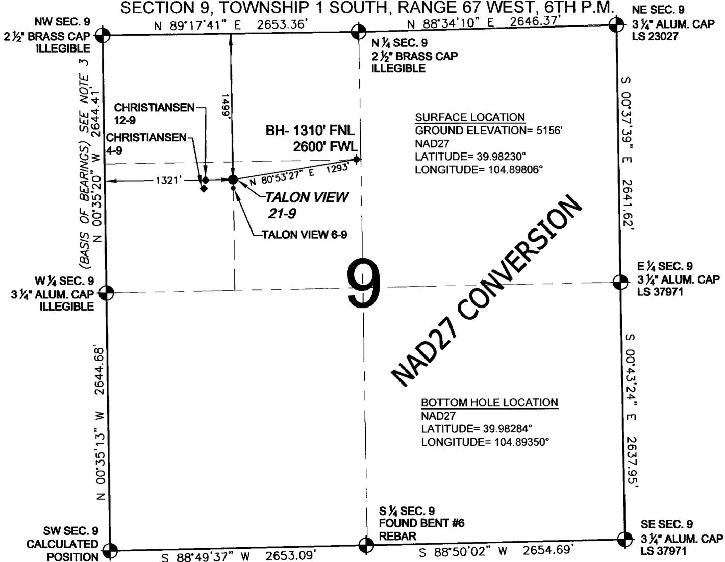
WELL TALON VIEW 21-9 TO BE LOCATED 1499' FNL AND 1321' FWL, SECTION 9, T1S, R67W OF THE 6th P.M.
