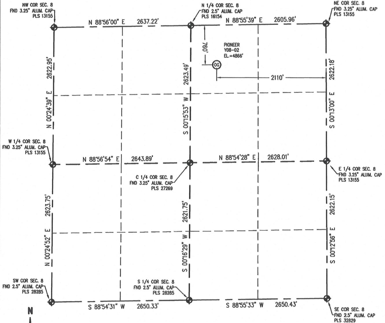
IN ACCORDANCE WITH A REQUEST FROM ERIK VAN DECAR - NOBLE ENERGY INC, BASELINE ENGINEERING CORP. HAS DETERMINED THE LOCATION OF THE PIONEER Y08-02 TO BE 760' FNL, 2110' FWL, AS MEASURED AT NINETY (90) DEGREES FROM THE SECTION LINE OF SECTION 8, TOWNSHIP 2 NORTH, RANGE 64 WEST, 6TH PRINCIPAL MERIDIAN, WELD COUNTY, COLORADO.
