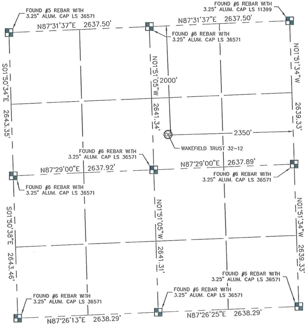
In accordance with a request from Dan Casper with Noble Energy Inc. King Surveyors Inc. has determined the surface location of the WAKEFIELD TRUST 32-12 to be 2000' from the NORTH line and 2350' from the EAST line as measured at right angles from the section line of Section 12, Township 2 South, Range 45 West of the Sixth Principal Meridian, County of Yuma, State of Colorado.
