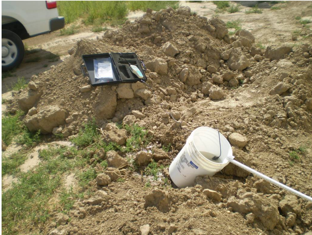
Photo #3 View of the purging process while recording parameters
