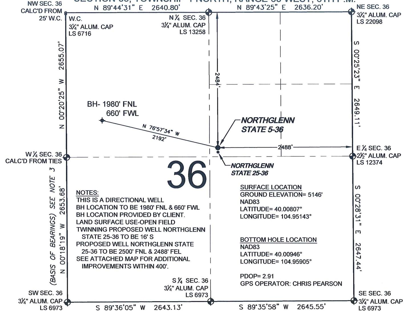
WELL NORTHGLENN STATE 5-36 TO BE LOCATED 2484' FNL AND 2488' FEL, SECTION 36, T1N, R68W OF THE 6th P.M.
