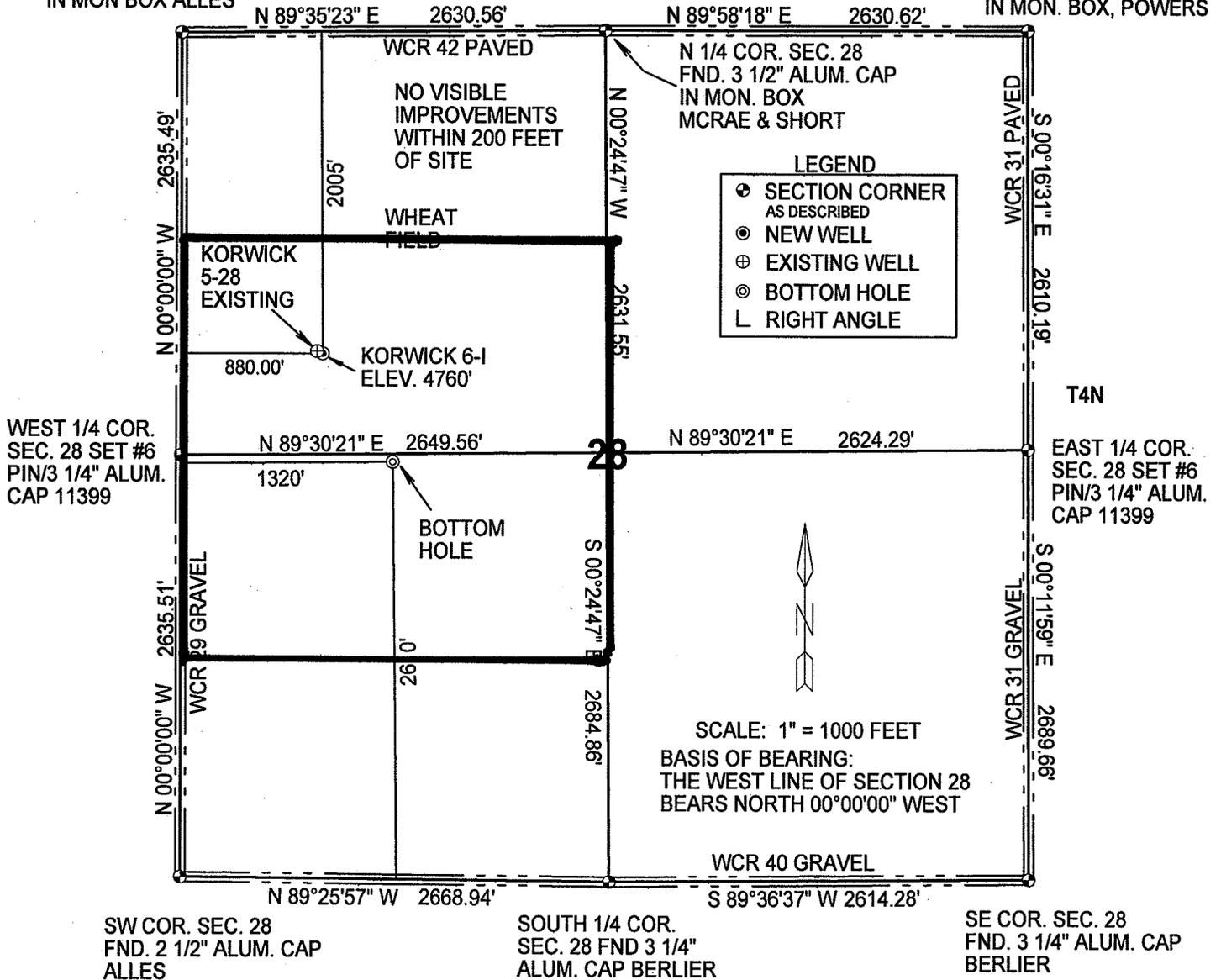
IN ACCORDANCE WITH A REQUEST FROM MERIT ENERGY COMPANY, THE UNDERSIGNED HAS DETERMINED THE LOCATION OF THE KORWICK 6-1 WELL TO BE 880' FWL AND 2005' FNL, SECTION 28, TOWNSHIP 4 NORTH, RANGE 66 WEST OF THE 6TH PRINCIPAL MERIDIAN, WELD COUNTY, COLORADO. FIELD SURVEY DATE: AUGUST 20, 2008
