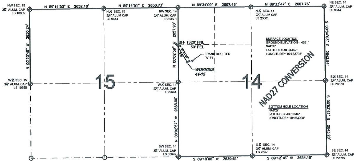
WELL WORRIES 41-15 TO BE LOCATED 1952' FNL AND 318' FWL, SECTION 14, T4N, R65W OF THE 6TH P.M.
