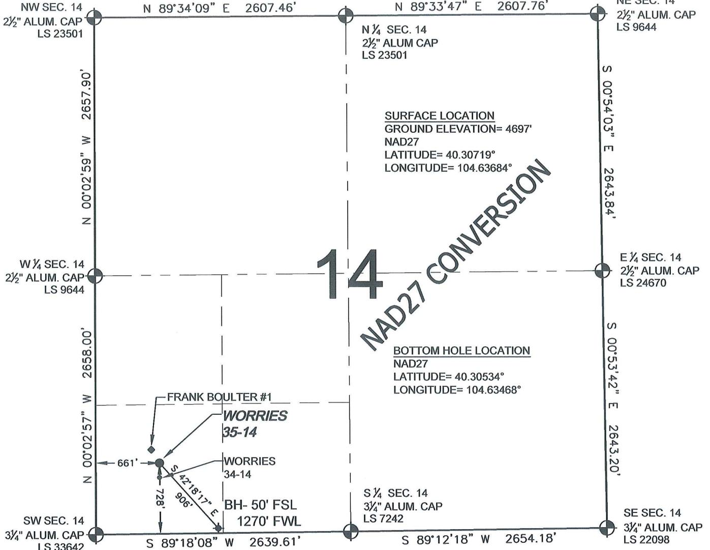
WELL **WORRIES 35-14** TO BE LOCATED 728' FSL AND 661' FWL, SECTION 14, T4N, R65W OF THE 6th P.M.
