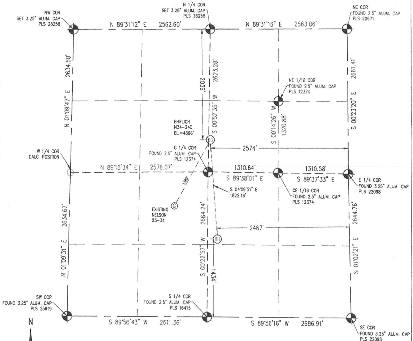
IN ACCORDANCE WITH A REQUEST FROM JOE MARTIN - NOBLE ENERGY INC, BASELINE ENGINEERING CORP. HAS DETERMINED THE LOCATION OF THE EHRLICH N34-240 TO BE 2036' FNL, 2574' FEL, AS MEASURED AT NINETY (90) DEGREES FROM THE SECTION LINE OF SECTION 34, TOWNSHIP 5 NORTH, RANGE 67 WEST AND THE BOTTOM HOLE LOCATION TO BE 1434' FSL AND 2467' FEL OF SECTION 34, TOWNSHIP 5 NORTH, RANGE 67 WEST, 6TH PRINCIPAL MERIDIAN, WELD COUNTY, COLORADO
