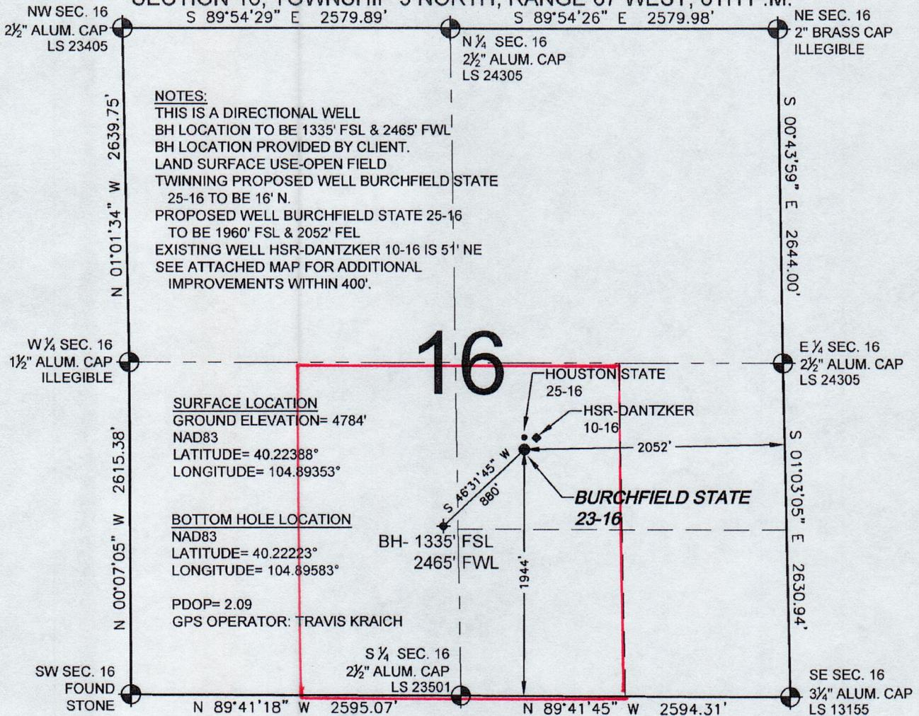
WELL BURCHFIELD STATE 23-16 TO BE LOCATED 1944' FSL AND 2052' FEL, SECTION 16, T3N, R67W OF THE 6th P.M.
