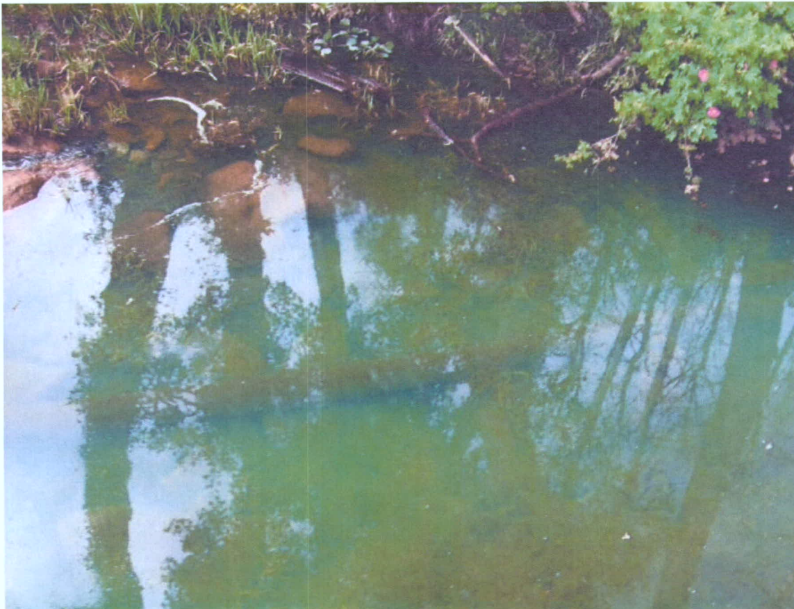
Photo 2- Tracer dye emanating from point source of Rock Spring
