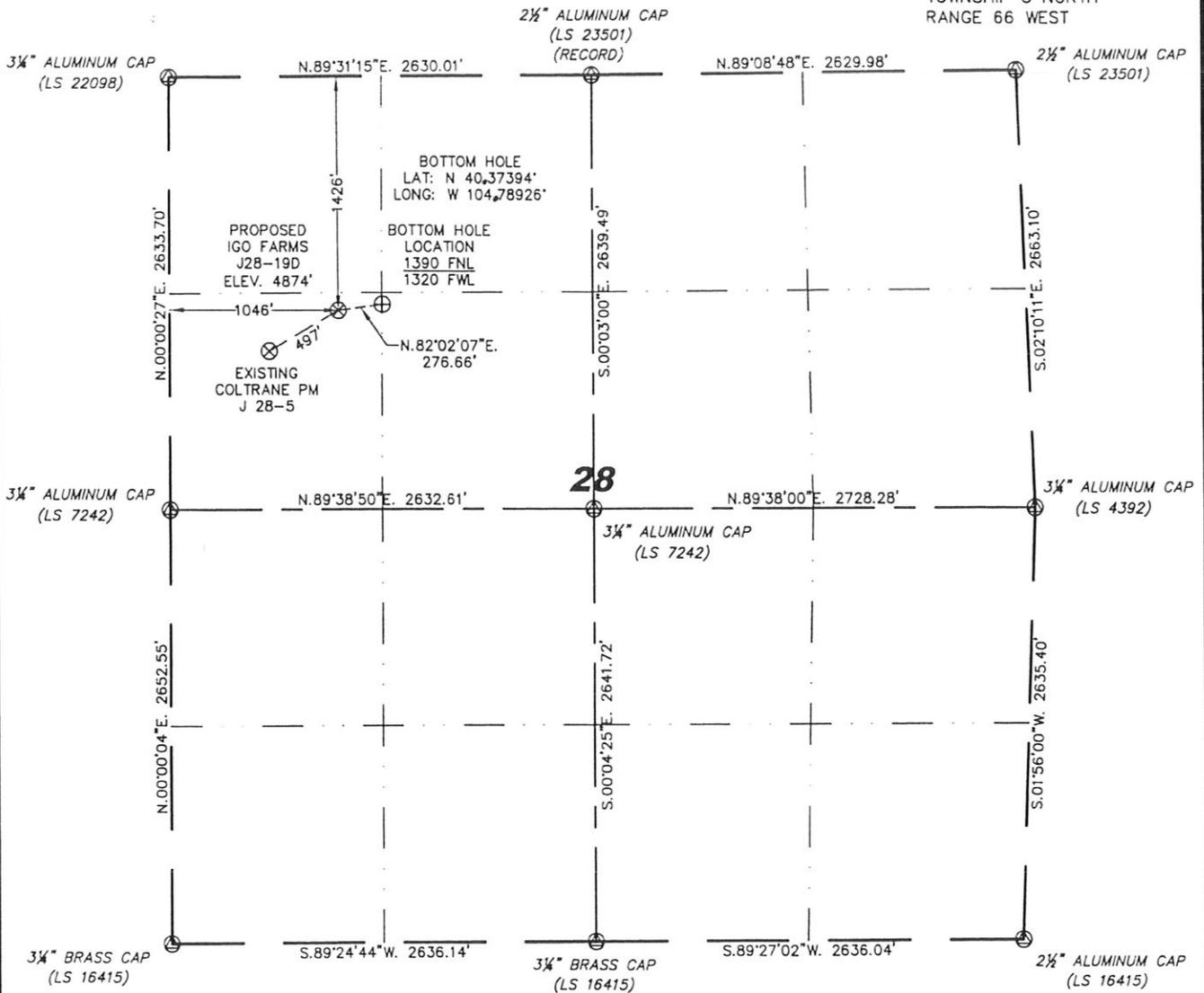
IN ACCORDANCE WITH A REQUEST FROM JACK FINCHAM - NOBLE ENERGY INC, STEIL SURVEYING SERVICES, LLC HAS DETERMINED THE LOCATION OF THE IGO FARMS J28-19D WELL TO BE 1426' FNL, 1046' FWL, AS MEASURED AT NINETY (90) DEGREES FROM THE SECTION LINES, SECTION 28, TOWNSHIP 5 NORTH, RANGE 66 WEST, 6TH PRINCIPLE MERIDIAN, WELD COUNTY, COLORADO.
