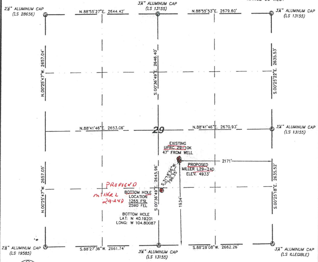
IN ACCORDANCE WITH A REQUEST FROM JOE JOHNSON - NOBLE ENERGY INC, STEIL SURVEYING SERVICES, LLC HAS DETERMINED THE LOCATION OF THE MILLER L29-240 WELL TO BE 1934' FSL, 2171' FEL, AS MEASURED AT NINETY (90) DEGREES FROM THE SECTION LINES, SECTION 29, TOWNSHIP 3 NORTH, RANGE 66 WEST, 6TH PRINCIPLE MERIDIAN, WELD COUNTY, COLORADO.
