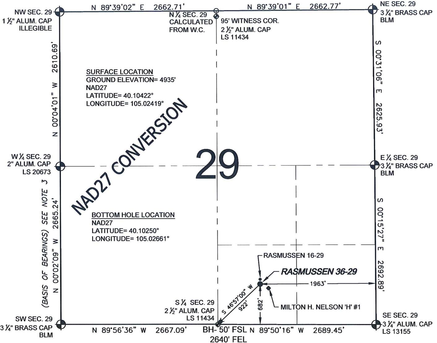
WELL **RASMUSSEN 36-29** TO BE LOCATED 682' FSL AND 1963' FEL, SECTION 29, T2N, R68W OF THE 6th P.M.
