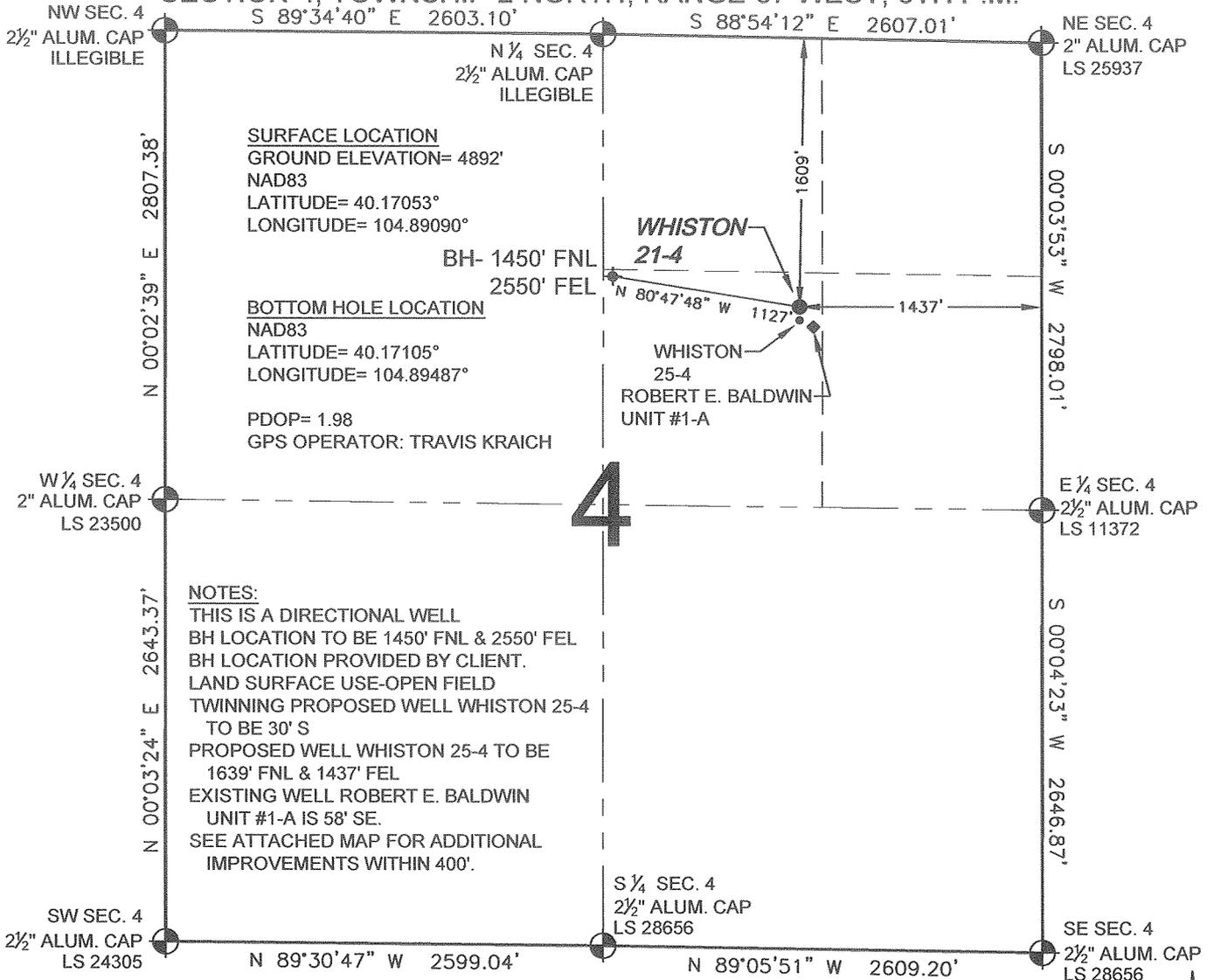
WELL WHISTON 21-4 TO BE LOCATED 1609' FNL AND 1437' FEL, SECTION 4, T2N, R67W OF THE 6th P.M.
