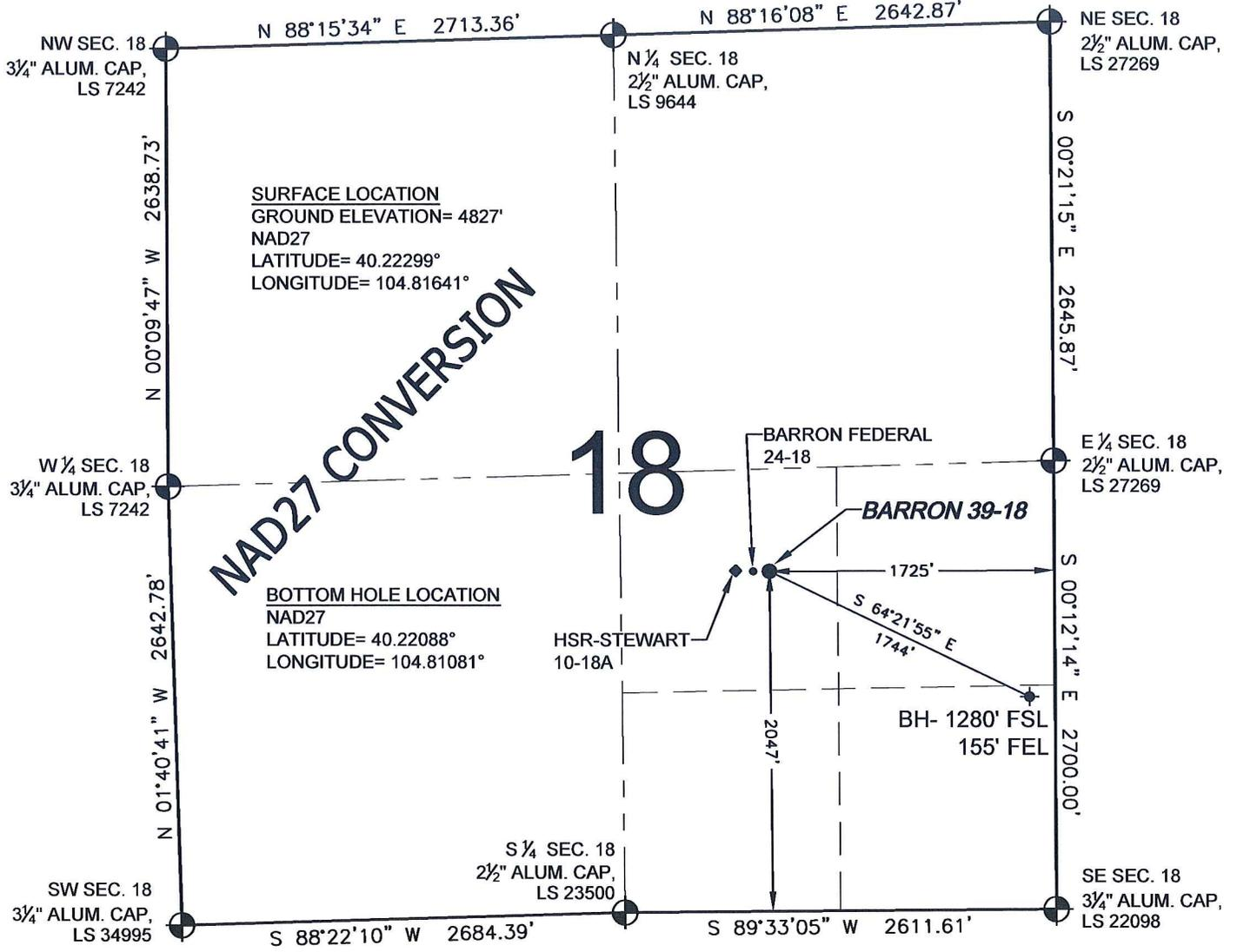
WELL **BARRON 39-18** TO BE LOCATED 2047' FSL AND 1725' FEL, SECTION 18, T3N, R66W OF THE 6th P.M.
