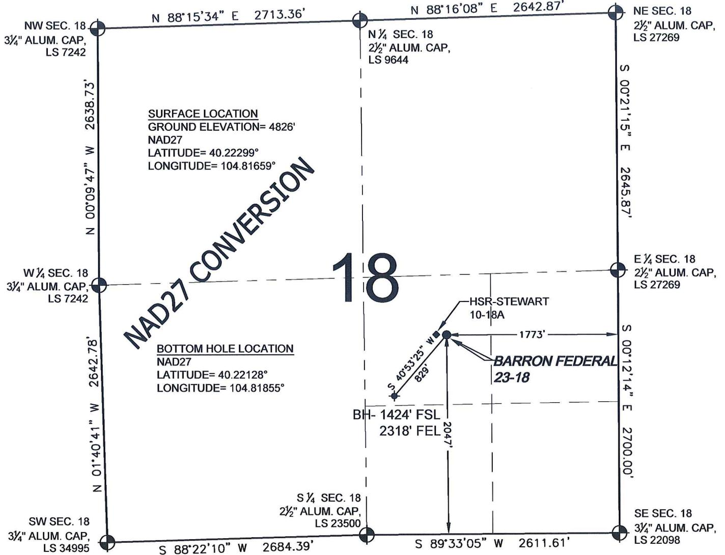
WELL **BARRON FEDERAL 23-18** TO BE LOCATED 2047' FSL AND 1773' FEL, SECTION 18, T3N, R66W OF THE 6th P.M.
