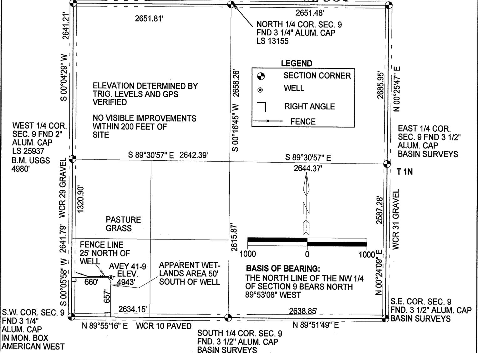
IN ACCORDANCE WITH A REQUEST FROM MERIT ENERGY COMPANY, THE UNDERSIGNED HAS DETERMINED THE LOCATION OF THE AVEY NUMBER 41-9 WELL TO BE 660' FWL AND 657' FSL, SECTION 9, TOWNSHIP 1 NORTH, RANGE 66 WEST OF THE 6TH PRINCIPAL MERIDIAN, WELD COUNTY, COLORADO. FIELD SURVEY DATE: FEBRUARY 6, 2007
