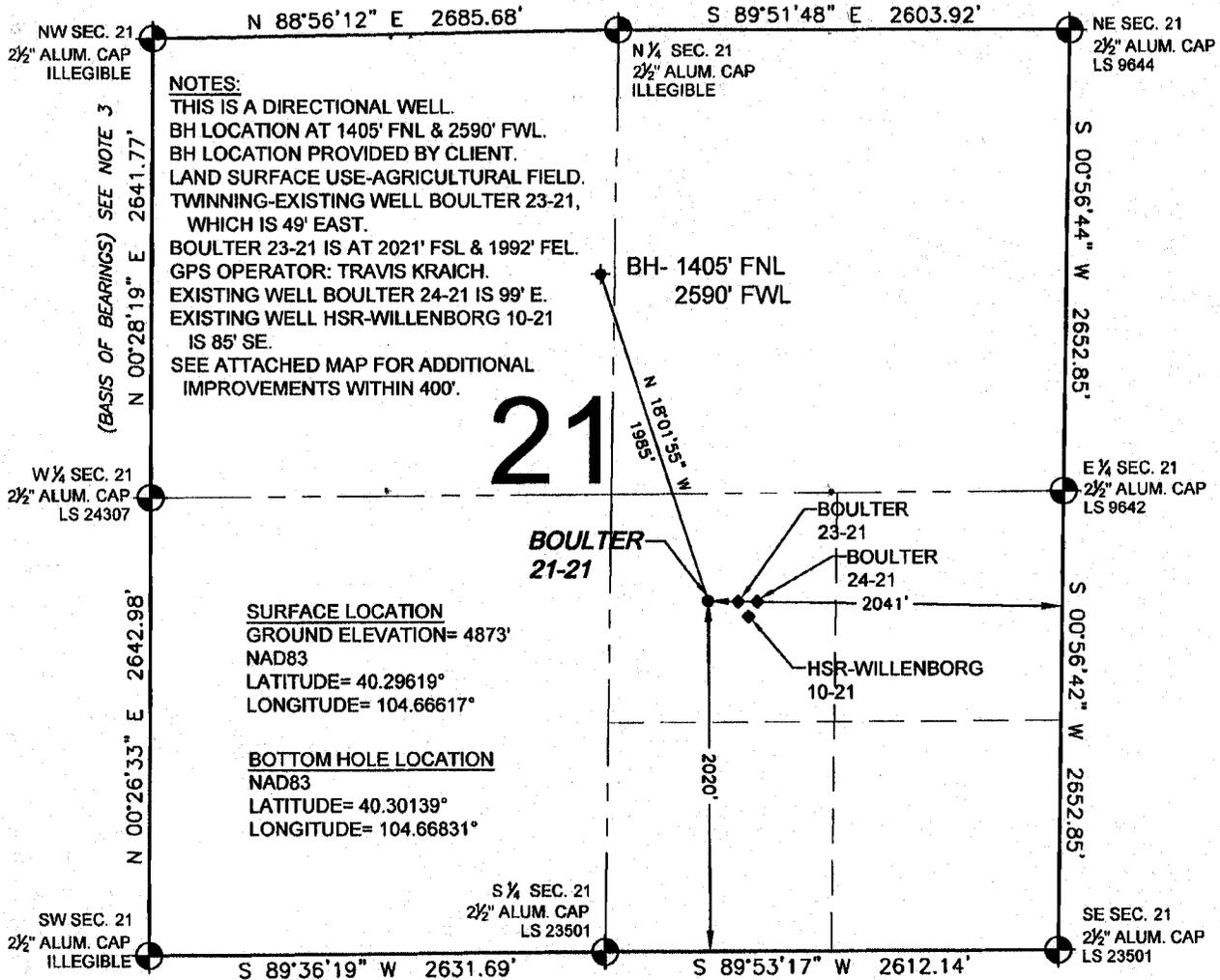
WELL BOULTER 21-21 TO BE LOCATED 2020' FSL AND 2041' FEL, SECTION 21, T4N, R65W OF THE 6th P.M.
