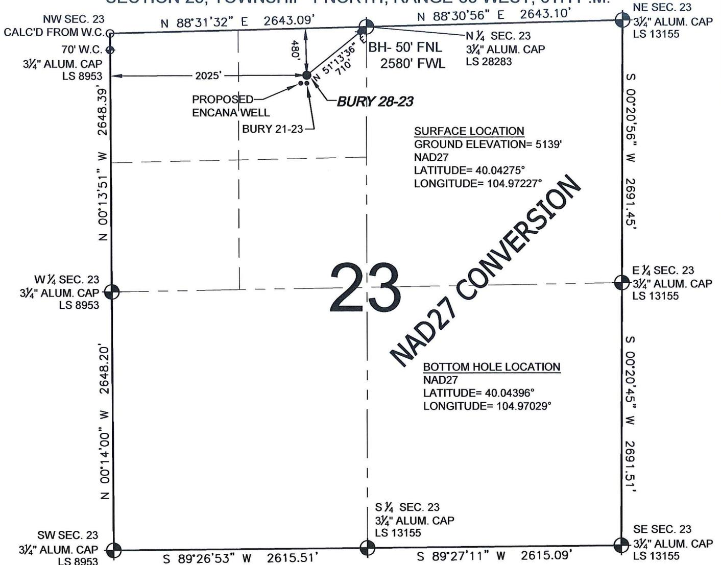
WELL **BURY 28-23** TO BE LOCATED 480' FNL AND 2025' FWL, SECTION 23, T1N, R68W OF THE 6th P.M.
