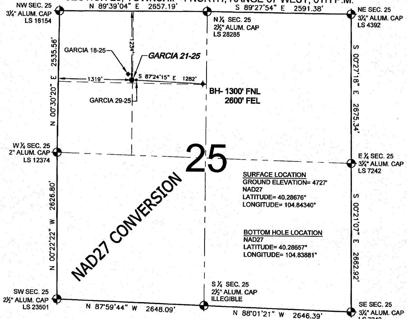
WELL GARCIA 21-25 TO BE LOCATED 1234' FNL AND 1319' FWL, SECTION 25, T4N, R67W OF THE 6th P.M.
