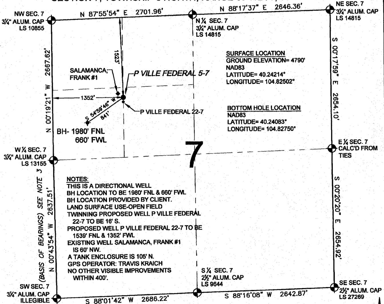
WELL P VILLE FEDERAL 5-7 TO BE LOCATED 1523' FNL AND 1352' FWL, SECTION 7, T3N, R66W OF THE 6th P.M.
