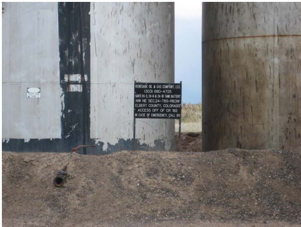
Photo 2. Two 300 BBL production tanks
