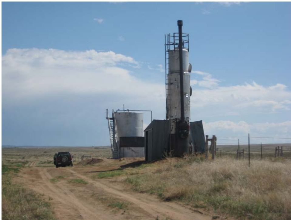
Photo 2. Vertical separator, fiberglass tank and battery tank
