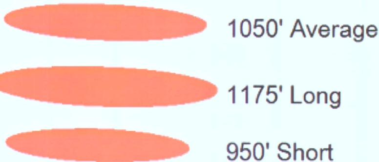
The image below shows drainage ellipses based on fracture half lengths of 1050' (average frac half lengths determined from the microseismic). This image demonstrates that gas reserves are left in the ground when the average drainage ellipse is used. Based on the frac lengths observed in Delta's microseismic program even the maximum frac half lengths of 1,175' leave gas reserves in the ground by only draining 16.6 acres.
