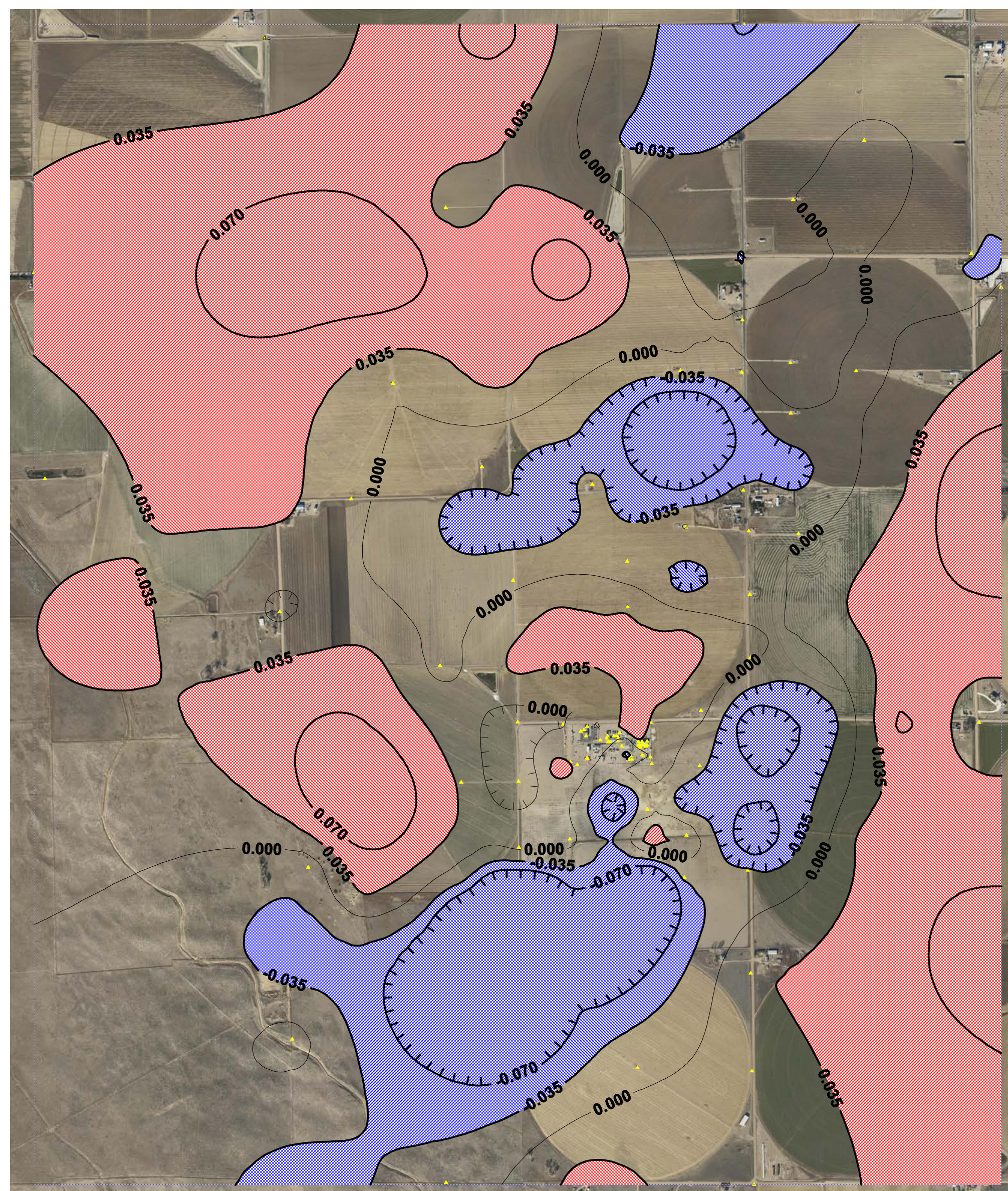
Cumulative Change in Benchmark Elevation (feet) Between 11-10-06 and 12-12-06
